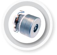
Series 498 vacuum cleaner motors are designed with an option to simultaneously drive a belt driven brush roll. Their skeletal construction has a diameter of 106 mm, and are available in a two-stage configuration. They can operate at lower RPMs and with a power of up to 1200 W, and are most commonly used in upright vacuum cleaners and low-power appliances.
