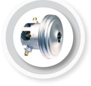
Series 462 vacuum cleaner motors for dry applications are mounted in a metal chassis. With their robust construction, they can be used for a broad spectrum of tasks. The external diameter of the chassis is 135 mm, with voltages from 100 V to 240 V and a maximum power of 2200 W. Their brushes can be replaced, enabling a highly affordable extension of their life-span. These motors are characterised by their reliability and the tried and proven materials.
